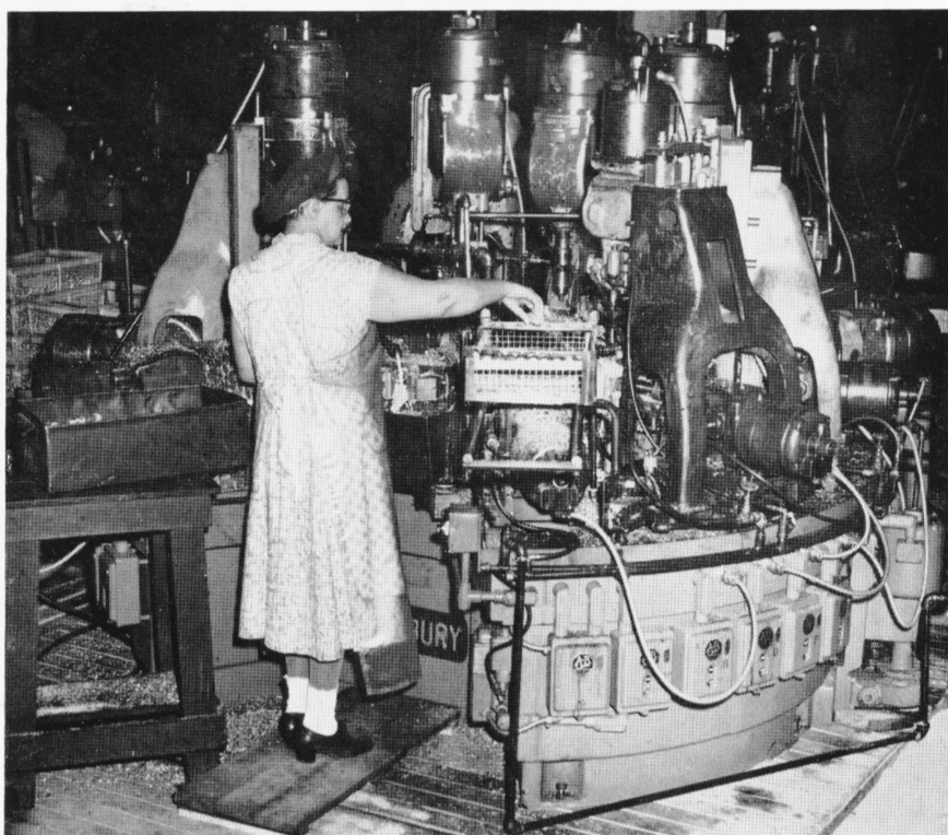
Anna Opel, Chucking, places a brass forging in the automatically operated chucks on a Kingsbury machine. She presses a button which indexes the machine and 27 operations are performed simultaneously.
